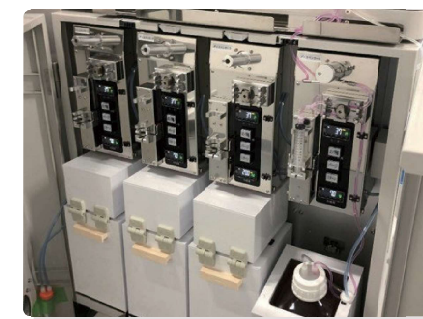
Four cooling units for medium storage
